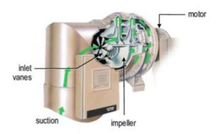
changing kinetic energy to pressure energy by centrifugal force
