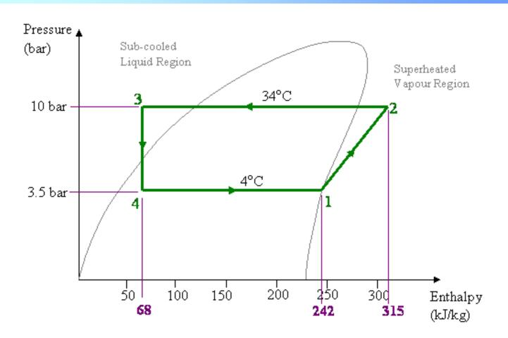
p-H Diagram of Refrigeration Cycle for 134a
